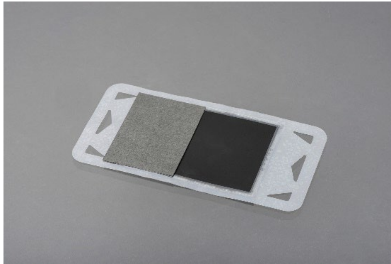
Figure 7: Photo of a MEA with half-laid GDL (light gray) on the CL (black) with reinforcement frame (white) (Source: FCI Fuel Cell Industrialization GmbH)
