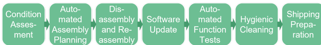
Figure 6: Planned refurbishment process chain for the second-life washing machine (Source: Miele)
